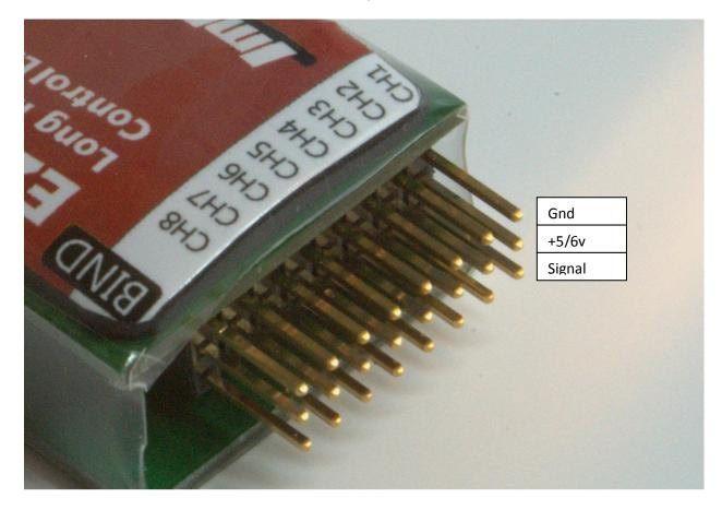
Servo connectors on the 8 channel receiver have the pin-out shown below.
