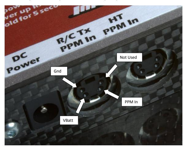
To remove any confusion, the pin-out is marked directly on a photo of the transmitter below:
