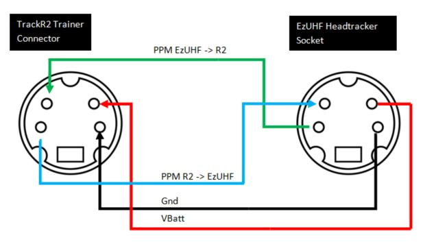
NOTE: The second PPM line is not actually required, but connecting it ensures that the cable can be connected either way around.
