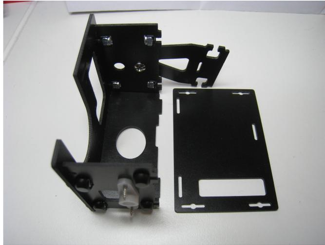
Finally, screw the servo horn to the servo.
