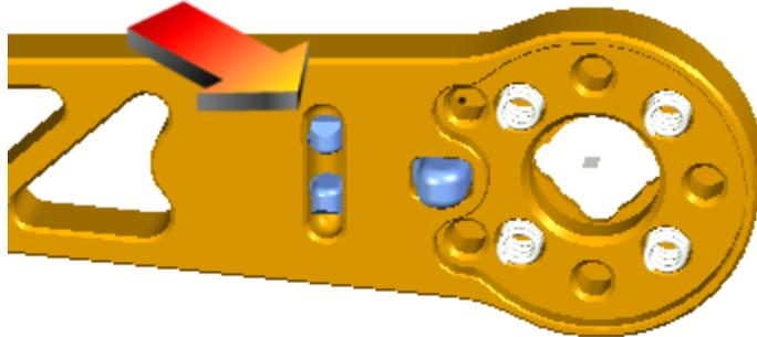
Warning: When the part is released, ensure that the spring, which is sandwiched between the arm and the white plastic part, doesn't 'boing' into the middle of next week!
