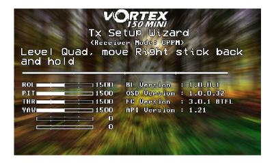
NOTE: To restart the wizard at anytime, power up the quad, press and hold the button on the led board until vortex beeps 2 times (first beep after ~3 seconds, second beep after ~5 seconds). Alternatively you can also enter tx Wizard via OSD menu
