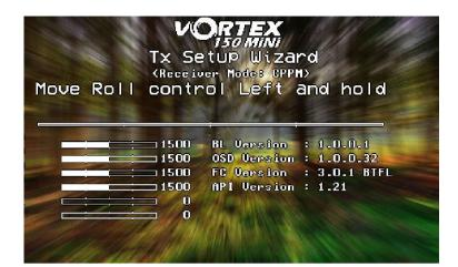
Follow the prompts, ensuring that the correct stick is moved each time. As each control is recognized, it's name will appear to the left of the servo bar.
