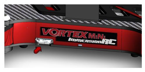
Please be careful not to put too much strain on this connector. It is a lightweight surface-mount part, and if the quad is dragged around by the USB cord it may not survive.
