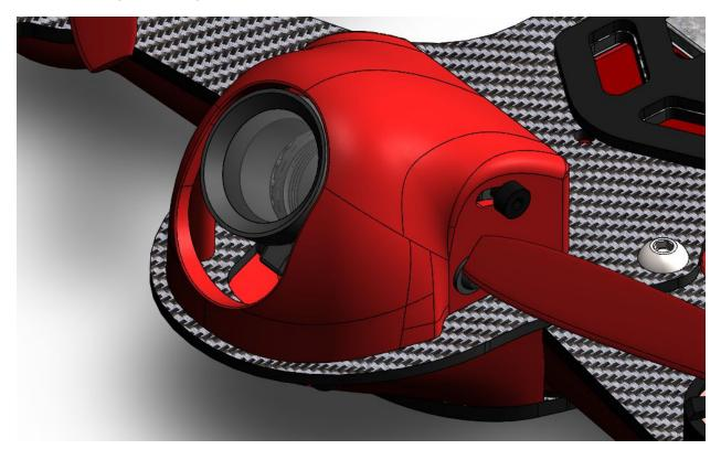
To remove the camera, simply remove the two hex-head screws under the nose of the quad and tilt the camera shroud upwards.
