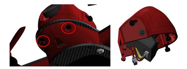
Note that the camera tilt is adjustable. Loosen the two upper-screws and tilt the camera to the desired angle, before re-tightening them.
