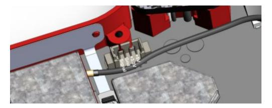
Note that a piece of double-sided tape may be used to secure the receiver on top of the metal can beside the connector.
