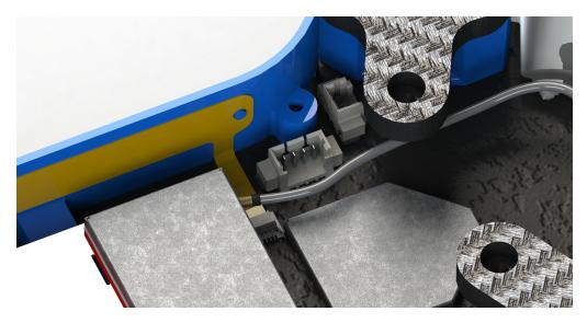
Finally, the receiver antennas may be routed through the two notches in the bottom of the LED diffuser or the two notches in front of the rear arms in the side-plates, which is the preferred configuration. Make sure you apply some extra shrinkwrap to the fragile antenna wires to make sure they put up with some abuse from rough landings and crashes as well as handling the mini-quad.
