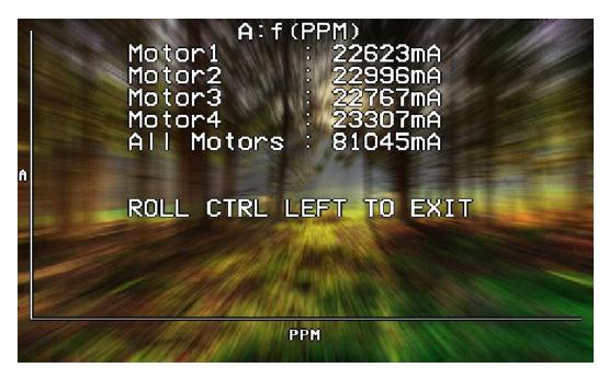
To exit the test move the Roll stick to the left.
