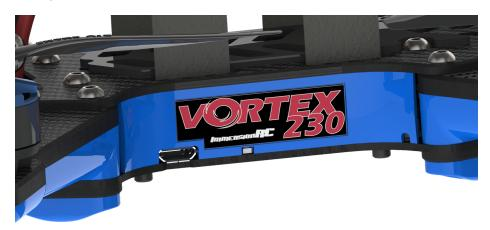
Please be careful not to put too much strain on this connector. It is a lightweight surface-mount part, and if the quad is dragged around by the USB cord it may not survive.
