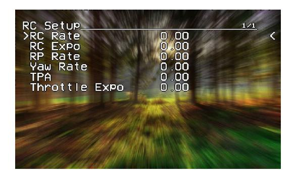
Note that all of the Flight Controller parameters can be preset by loading one of the installed <u>Pro-Tunes</u>.
