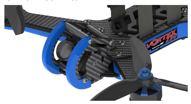
Note that the camera tilt is adjustable. Loosen the two upper-screws and tilt the camera to the desired angle, before re-tightening them.
