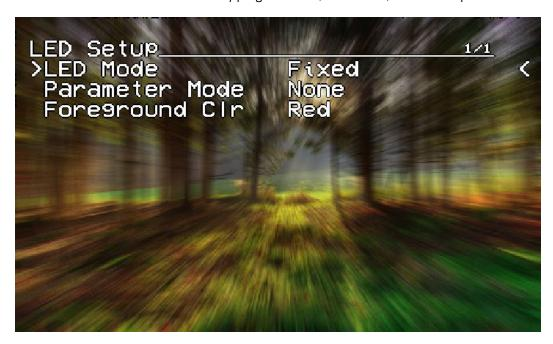
For Parameter Mode = **Intensity**, the intensity of the LEDs will reflect the current throttle position.
