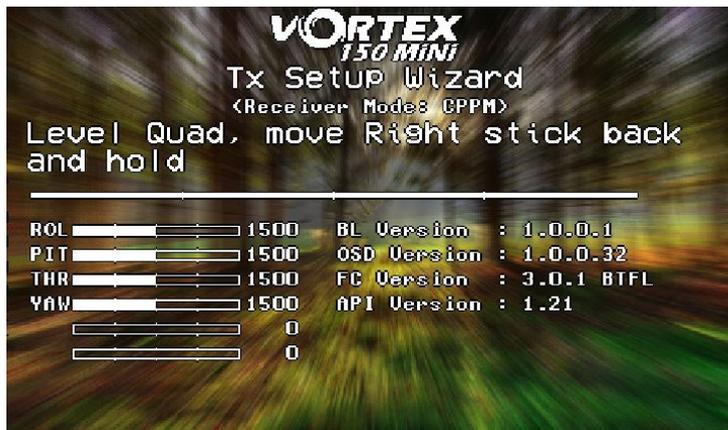
*NOTE: To restart the wizard at anytime, power up the quad, press and hold the button on the led board until Vortex beeps 2 times (first beep after ~3 seconds, second beep after ~5 seconds). Alternatively you can also reset the Tx Wizard via OSD menu*
