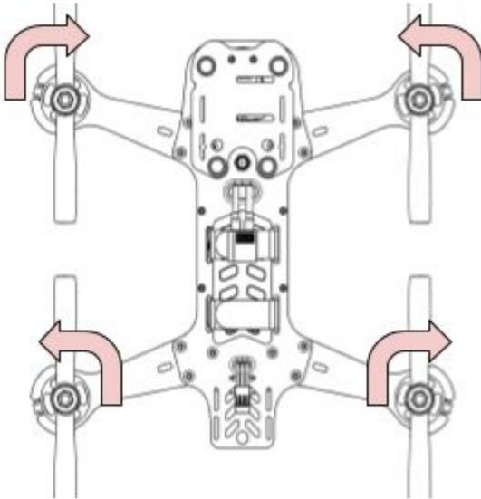
**P.S. To arm the flight controller after running the wizard, for mode 2, move the throttle stick down and to the right. See 'Flight Controller Stick Commands' in the main manual.**
