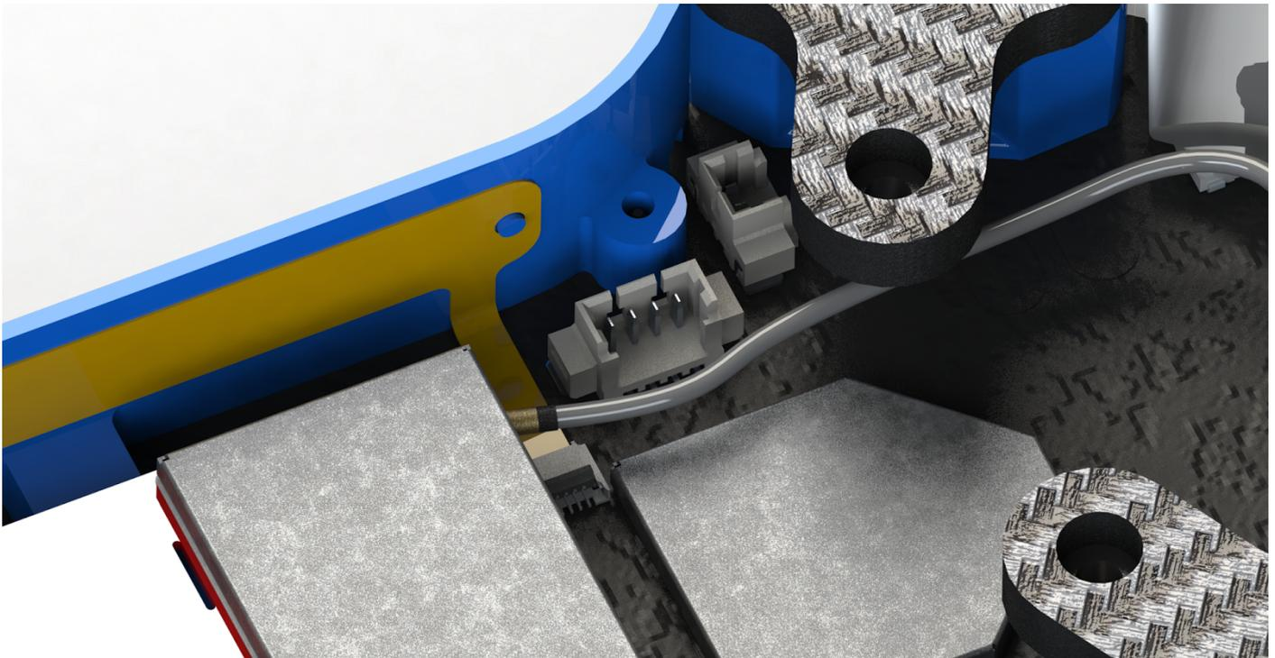
Finally, the receiver antennas may be routed through the two notches in the bottom of the LED diffuser, or through the two notches in front of the two rear arms, which is the preferred solution. Make sure you apply some extra shrinkwrap to the fragile antenna wires to make sure they put up with some abuse from rough landings and crashes as well as handling the mini-quad.
