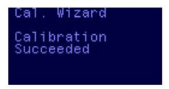
If the calibration procedure fails, then it is like due to one of two causes. The first is that the selected channel was not 'empty' when the first part of the calibration was attempted. The second is that the selected channel did not have a transmitting vTx when the second part of the calibration was attempted.
