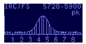
An interesting point to note in the Spectrum Analyzer is that the channels for each selected band are shown under the graph. For the rarely used bands E, B, and A, the rather odd frequency mapping is clearly visible when switching between the bands.
