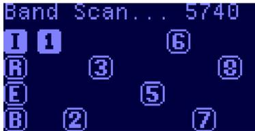
To enter into the band scanner you can either hold down the joystick on the main screen, or select 'Band Scan' from the tools menu.
