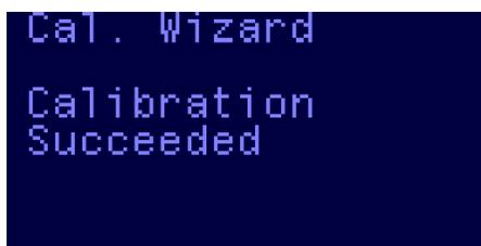
If the calibration procedure fails, then it is likely due to one of two causes. The first is that the selected channel was not 'empty' when the first part of the calibration was attempted. The second is that the selected channel did not have a transmitting vTx when the second part of the calibration was attempted.
