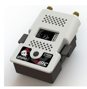
If only one antenna is available, the **Antennas** menu may be used to configure which antenna (or both) is used. < for the left antenna, > for the right antenna, and <> for both.
