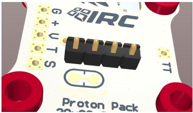
2) Install the Tramp Nano/Ghost on the correct side of the board, until it is touching the Proton Pack. For the Tramp, a small dab of thermal paste on the two black ICs that will touch the Proton Pack will improve thermal performance (this is available from any computer store).
