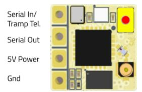
Note that the antenna connector on the Zepto is an MHF4, and not a standard U.FL.
