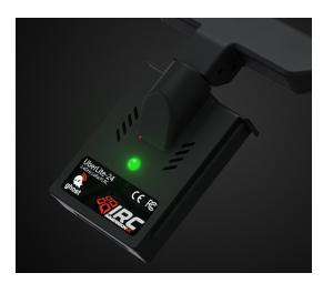
To Update the UberLite module, press and hold the lit **Bind** button while powering up the remote.
