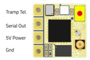
Note that the antenna connector on the Zepto is an MHF4, and not a standard U.FL.
