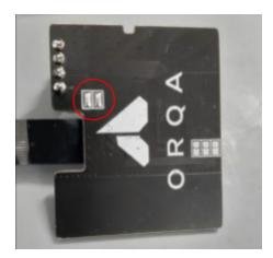
3. Connect the FPV.Connect antenna and Ghost Rx antenna connector with small U.FL to U.FL cable.
