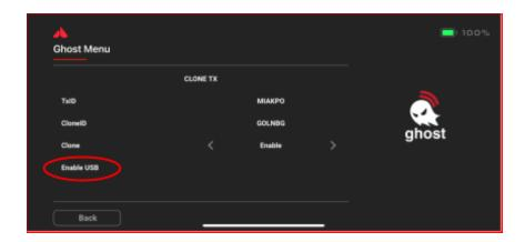
Once the slave has been written, it will inherit the Master's ID, and may be used interchangeably with the Master radio, without the need to rebind receivers.
