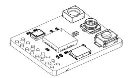
Note: For the Atto v1 and Atto v2 (July 2022) a power supply of 5V is required. For the v1, exceeding 6.5V can damage the receiver. For the v2, this is raised to more than 10V before damage occurs.
