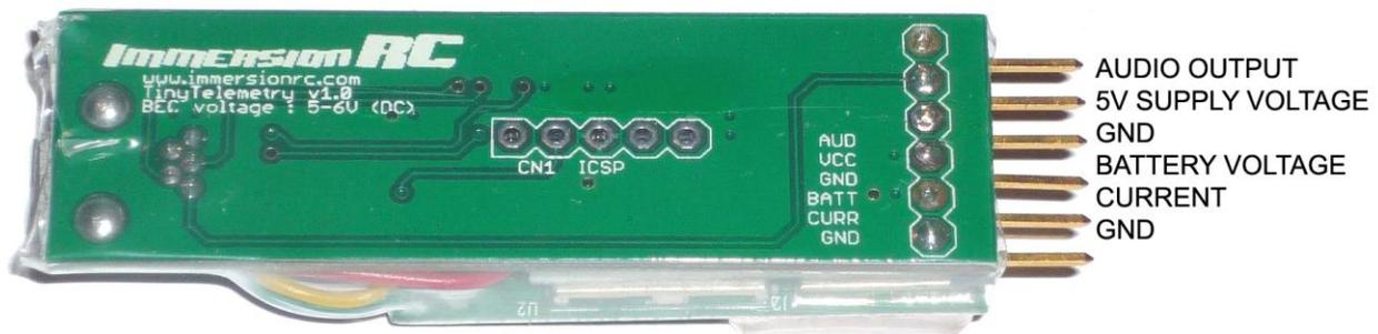
The bottom three pins are labelled 'battery voltage', 'current' and 'gnd'. Battery voltage allows monitoring of the flight pack battery voltage. Route this pin to the positive terminal (+) of the battery pack. If current sensing isn't required no other connections need to be made.
